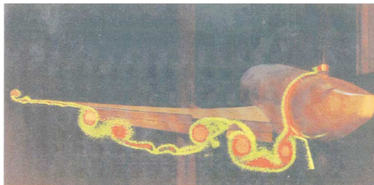
Fig. 1. Complex environment behind a wing illustrated by pressure losses contour plot (after Crowder, 1980).
